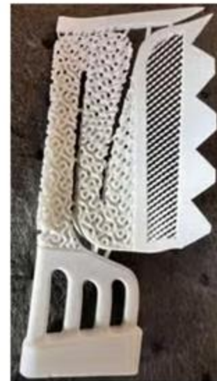
A ceramic 3D printed mold for Honeywell's turbine blades.
